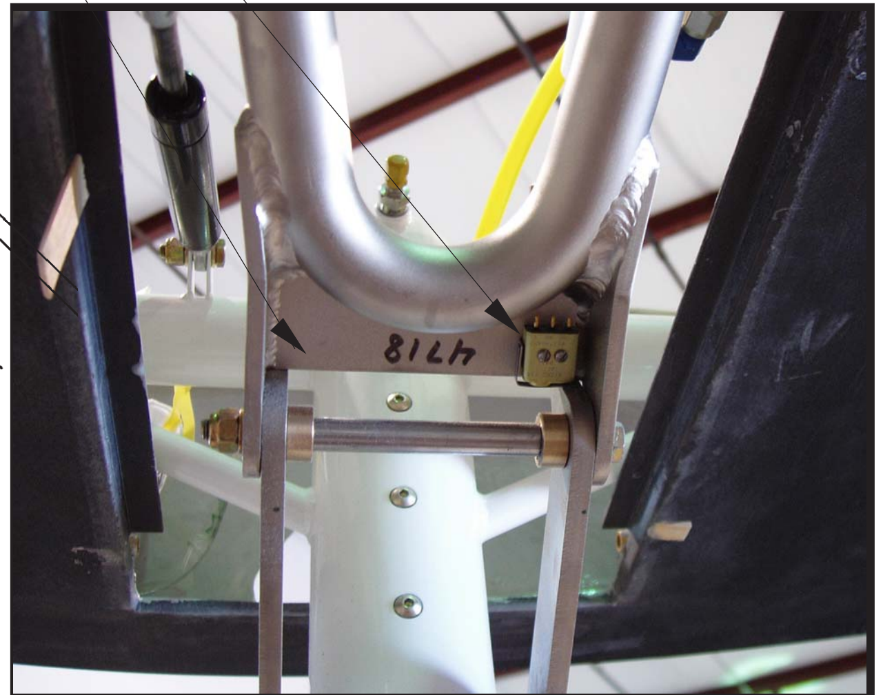
This photograph is taken from beneath the main gear, looking up at the switch.
